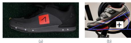
Figure 3. (a) Five markers were placed on each shoe. (b) Pedal-ground angle. Positive values (+) signify heel-up position (as shown in (b)), negative values (-) heel-down.
