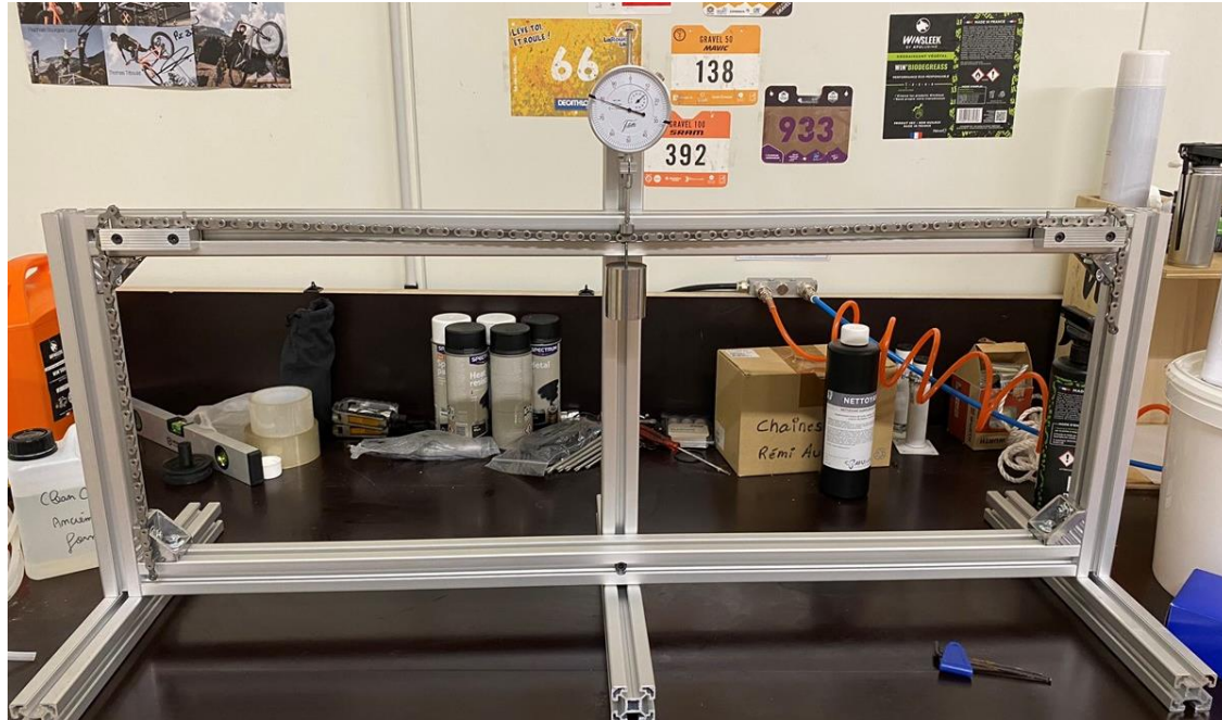
Chain elongation (precision 0.0005 mm) through chain sag
