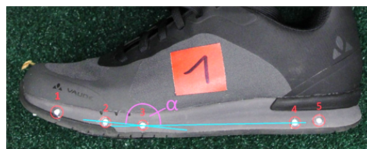
Figure 2. Test shoe with markers and the MTP-angle ( \alpha ).
