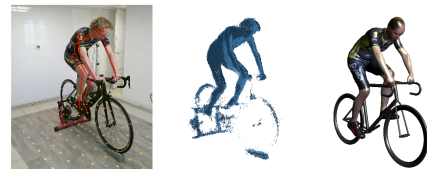
Data recording 3D point cloud and parametric model
