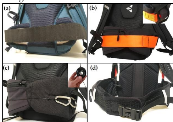
Figure 2. Belt conditions: (a) Elastic Band (EB), (b) Seatbelt (SB), (c) Spring balancer (SPRING5 & SPRING20), (d) Conventional Belt (CB).
