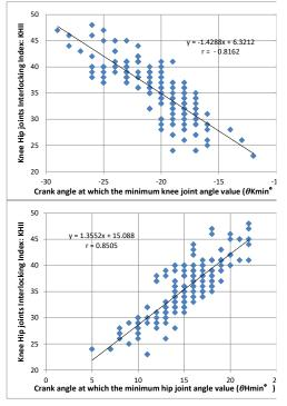
Figure 1. Relationship between the crank
