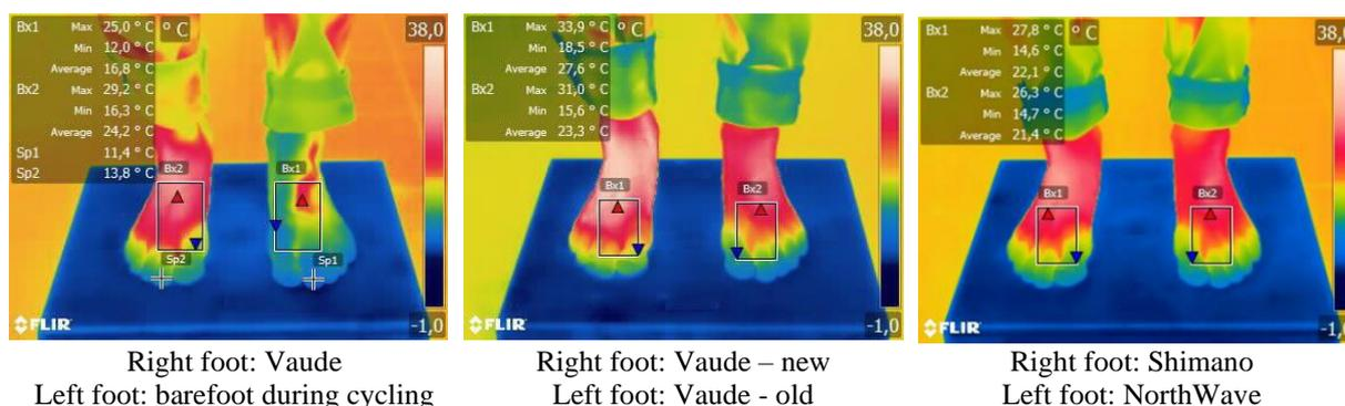
Figure 6. Thermal images of skin surface temperature (dorsal view; same subject); red colour illustrates warmer temperature, blue colder surface temperature
