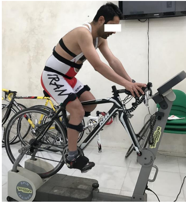
Figure 1: the depiction of a subject on the bicycle attached to Technogym ergometer and the location of myoMotion sensors on segments
