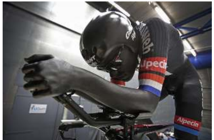
3D-printed mannequin in the wind tunnel
