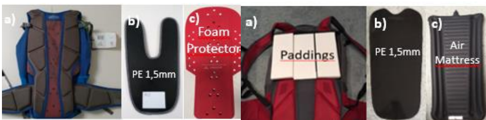
Fig. 2: Left: a) Moab Pro 22L; b) 1,5 mm thick polyethylene plate; c) Ortema foam protector (2 cm thick, weight 395 g and 50 Asker C). Right: a) Bracket 22 L with 10, 20 mm thick EVA foam paddings (20 Asker C); b) 1,5 mm thick polyethylene plate (PE); c) inflatable air mattress (3 cm thick, weight 200 g)
