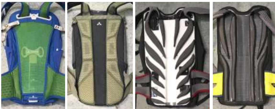
Figure 3. Rear panels of the tested backpack conditions; Left to right: Ventilated system (VS), full contact system (FC), AirTurbulencer concept (AT), AirStreamer concept (AS)
