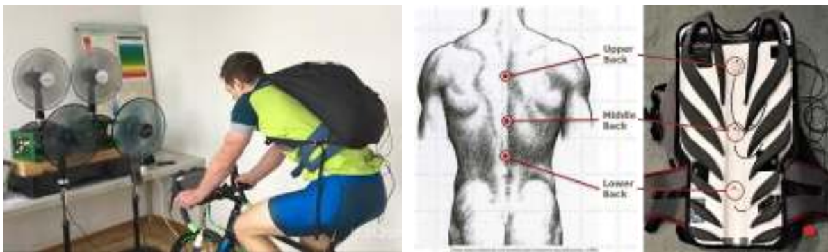
Figure 2. Left side: Test setup with 4 floor fans aligned with frontal upper torso; Right side: Sensor position on the back and the backpack
