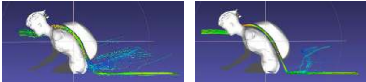
Figure 3. Cross section view along sagittal plane of body centre: Colour pattern indicates airstream velocity (red: high velocity; blue low velocity) and turbulences (left side: AirStreamer concept; right side: AirTurbulencer concept)
