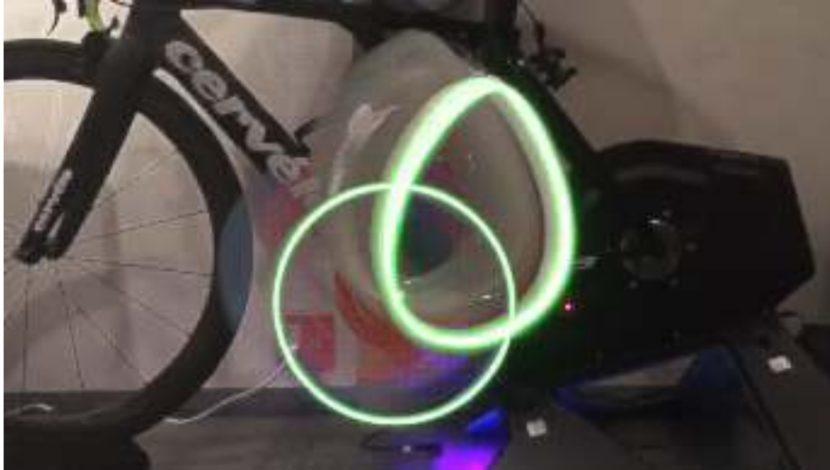
Fig 2. Pedal axle and heel movement (1min, 200W)
