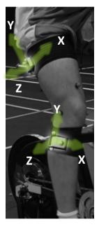
Figure 1 Sensor positioning on thigh and shank and local axis
