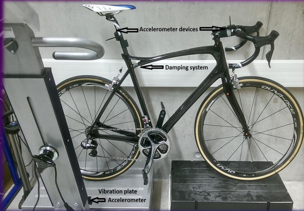
Figure. Experimental set-up (bike without the cyclist)
